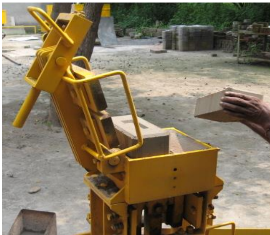
Step-7: Remove the blocks carefully and place it on the wooden tray. Move the lever and the yoke at the initial position.
