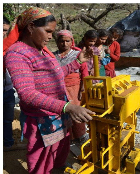
Close the mould lid with an impact using the lever handle and engage the lock.
