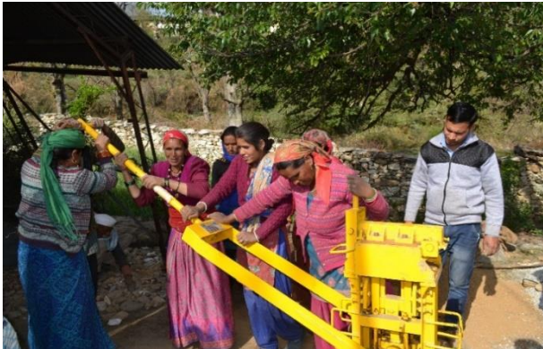
Raise the lever and yoke by 1 inch, disengage the lock and open the mould lid. Move the lever below the horizontal plane till the entire block and part of ram plate comes out of mould.
