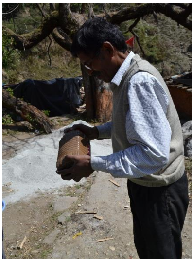
Mix soil and water in a transparent jar and shake it well
