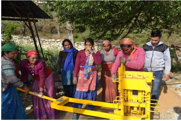
On the compaction side, 'press' the lever till it rests on the ejection pivots.
