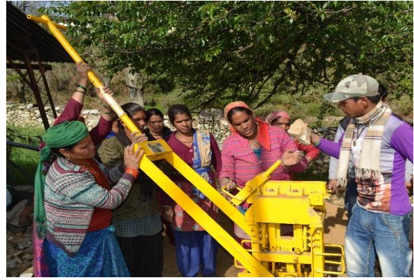
On the compaction side, 'press' the lever till it rests on the ejection pivots.
