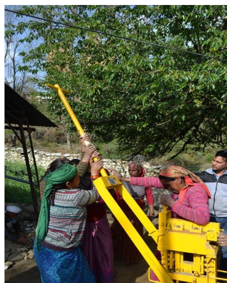
Move (throw) the lever and yoke to the compaction side.
