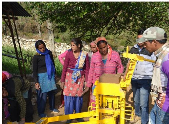
Remove the blocks carefully and place it on the wooden tray. Move the lever and the yoke at the initial position.
