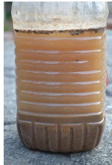
Check the layers after sedimentation process
