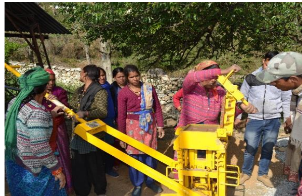
Raise the lever and yoke by 1 inch, disengage the lock and open the mould lid. Move the lever below the horizontal plane till the entire block and part of ram plate comes out of mould.
