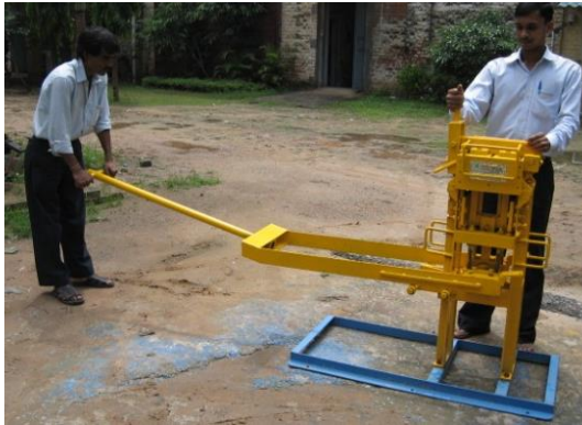
Step-5: On the compaction side, 'press' the lever till it rests on the ejection pivots.
