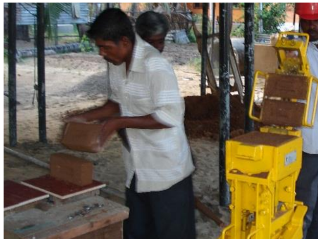
Step-7: Remove the blocks carefully and place it on the wooden tray. Move the lever and the yoke at the initial position.
