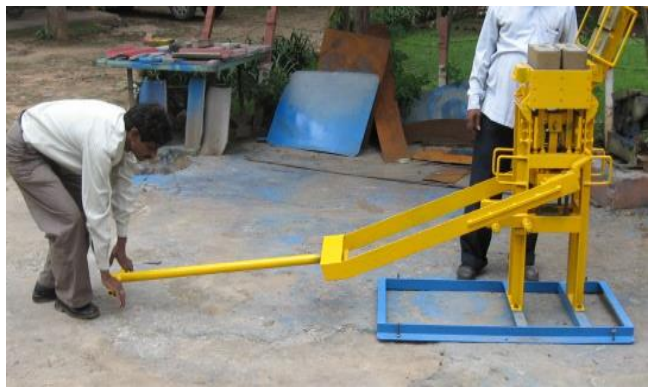
Step-6: Raise the lever and yoke by 1 inch, disengage the lock and open the mould lid. Move the lever below the horizontal plane till the entire block and part of ram plate comes out of mould.
