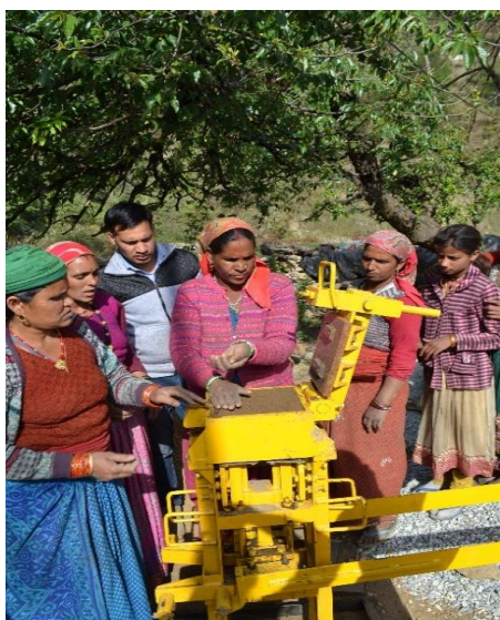
Fill prepared soil into the scoop and fill the mould. Take care the mould is filled to the top and level the surface.
